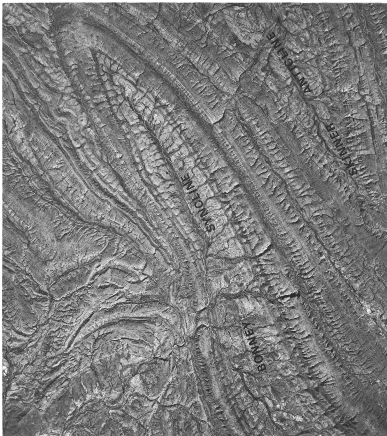
Fig. 3. Aerial photograph of central part of Davenport Province, showing NW-trending Bonney Syncline and Skinner Anticline of first folding episode, and NE-trending anticlines (upper and lower right) of second folding episode. Location of photo shown in Fig. 1(b). Width of field 14 km. Part of Bonney Well CAG 4112, Run 6, photo 0024, 1971. Crown copyright reserved.
